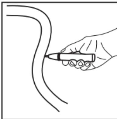
Voltage test at Insulated conductors
