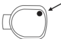
This point is marking the location of max. sensitivity for magnetic sensor..
